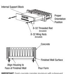
**IMPORTANT**: Fresh concrete corrodes aluminum with subsequent release of hydrogen. Concrete must be fully cured prior to installation of steplight to prevent any damage.
